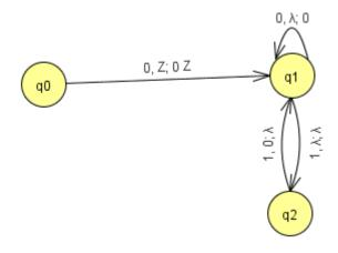
At this point, observe that whenever the automaton is in state  $q_2$  it has seen an odd number of 1s and whenever it is in state  $q_1$  it has seen as even number of 1s. If you recall building a DFA or an NFA to recognize a string with an even number (or odd number) of 1s, this should look familiar.
